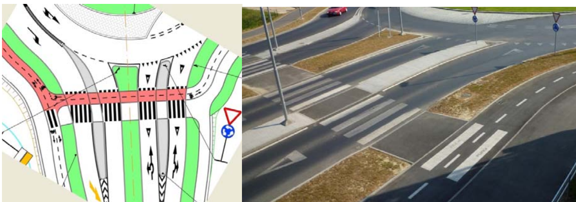
Figure 22. Arrangement of pedestrians and cyclists crossing in turbo roundabout in city Koper
